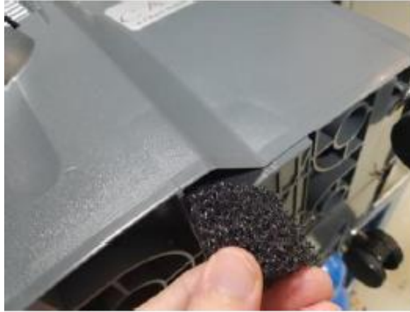
Figure 5. Required Bottom Gross Particle Filter. Located in front of compressor intake on bottom of unit.
