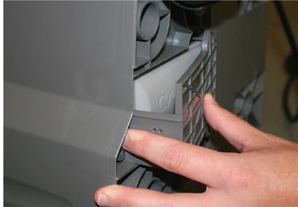
Figure 3. Air Intake Filter (cartridge). Located under filter cover.
