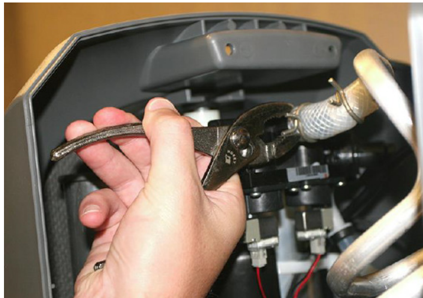
Fig. 4: Previous Design Clamp Removal
