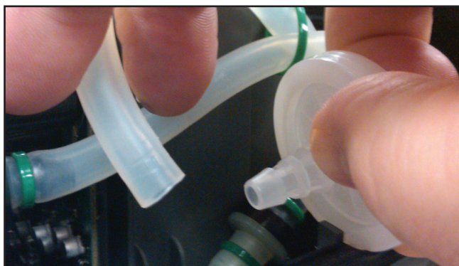
Figure 20: Disconnecting the HEPA Filter.
