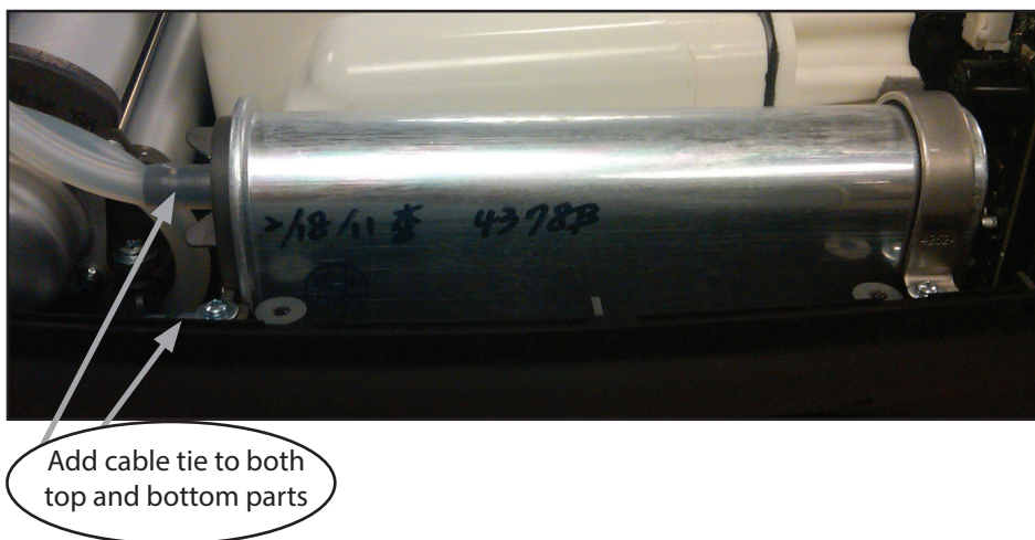
Figure 48: Connect output tubing
