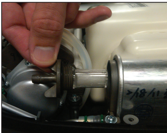
Figure 24: Unscrewing the HEPA Filter.
