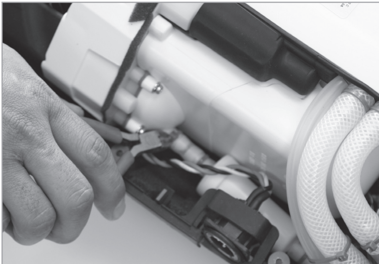
Figure 27: Removing the Compressor Intake Filter.
