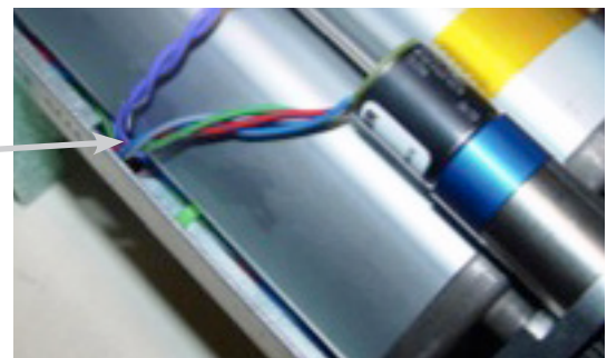
Figure 11-50. Route ATF wires
