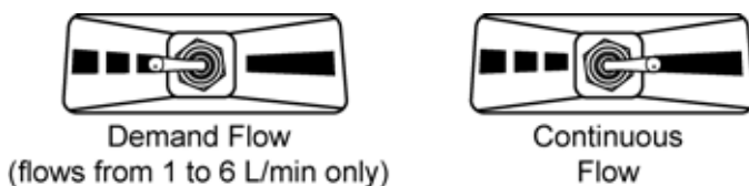
Figure 17: Continuous/Demand Flow Switch
