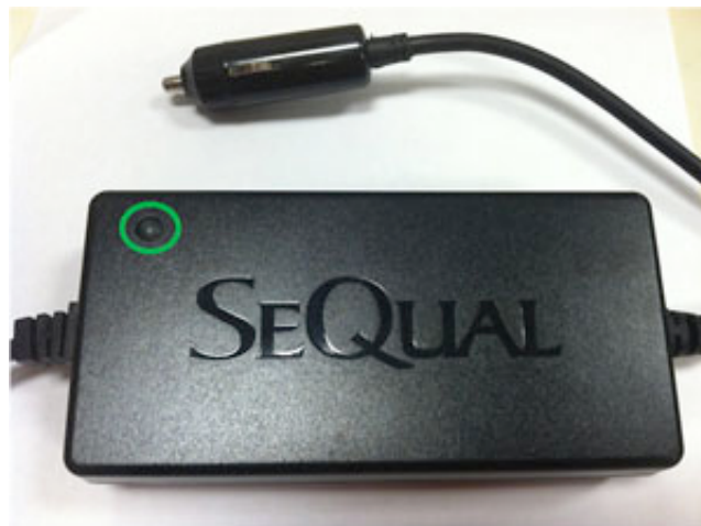
Green Status LED Location on the DC Power Supply
