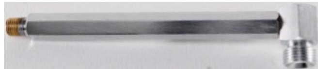
This is the elbow that attached to the flow control valve and serves as the oxygen outlet. It contains a DISS outlet. A humidifier bottle can be attached to this elbow, or a cannula can be directly attached using a DISS Adaptor (Christmas Tree) fitting.
