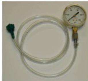
Attaching the gauge to the oxygen outlet and turning the flow control valve to a setting of 2.0LPM or higher will allow you to monitor the pressure inside the reservoir while filling.
