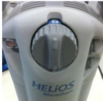
A: The HELiOS Marathon must detect a breath to begin delivering both demand and continuous flow. No flow will be delivered until a breath is sensed through the bottom cannula barb. A dual-lumen cannula must be connected to the Marathon and a patient must begin breathing before the flow will start.
