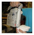
If the leaking continues even when the fill connectors are clean and dry, then the fill connector poppet is likely warped or
