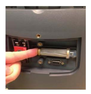
5. Once the 9-Volt Battery has been replaced, the next step is to replace the Compressor Intake Filter. To remove the Compressor
