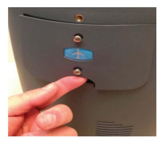
3. Once the cover is removed, replace the 9-Volt Battery by pushing
