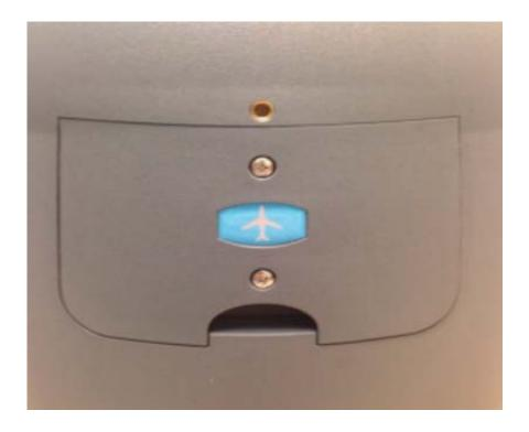
1. Remove the rear cover by loosening the two Phillips-head screws.
