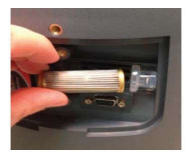
6. To insert the new Compressor Intake Filter, align the end of the filter with the inlet hole with the plastic housing on the eQuinox.
