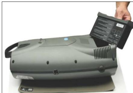
2. Place the Eclipse front side down on an approved ESD mat or work bench.
