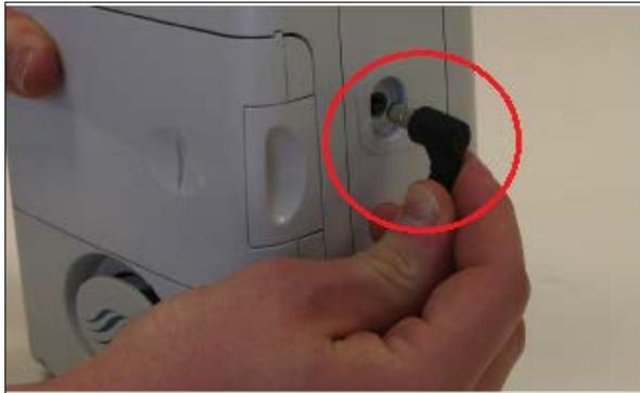
2. Connect the DC power cord to the inlet marked "ACCESSORY DC IN" on the universal power supply.
