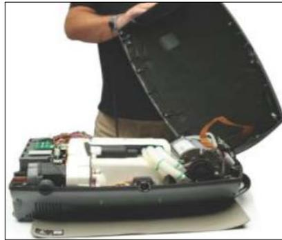
5. Remove the old 9V DC battery from the bottom of the unit and replace it with the new battery provided in the preventative maintenance kit. Use the foam adhesive tape, also provided in the kit, to secure the battery and prevent it from rattling inside the unit.
