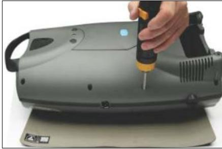
4. Turn the unit over onto its back and remove the front cover assembly. Be careful not to damage the control panel ribbon cable or the oxygen delivery tubing.
