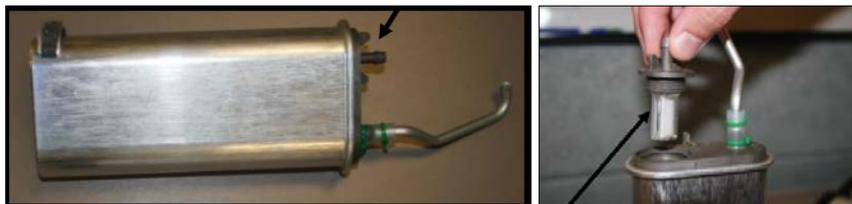
8. Remove the old compressor inlet filter and replace it with the new one provided in the preventative maintenance kit. Secure the filter with the zip ties provided in the kit. Be sure to pay attention to the direction of flow on the filter. The arrow on the filter should point down towards the bottom of the unit.
