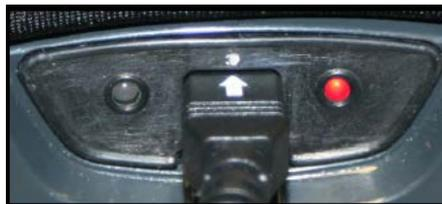
2. Within 2 seconds of the green LED staying on, power the unit off.
