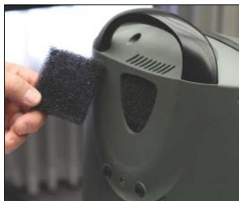
13. Clean the exterior of the unit with a damp cloth. It's recommended to use a mild solution of detergent and water when doing this. Do not expose the Eclipse to excess water. It may damage the unit.
