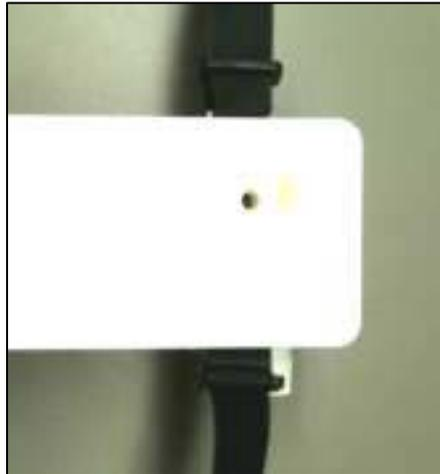
**Step 2.** Reverse the "nap" direction on the bottom hook and loop strap of the muffler assembly such that the hook and loop material faces up.
