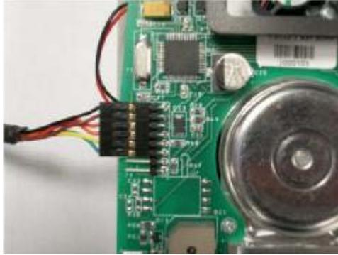
6. The Data Cable is now connecting the PC and the AirSep Focus. Next plug the AirSep Focus unit into AC power, and then put the unit into test mode.
