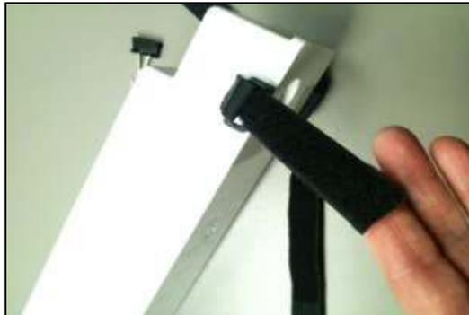
**Step 5.** Install the filter into the muffler assembly by securing the bottom strap to the hook and loop strip on the filter and then over top of the top strap. Ensure port on filter is not obstructed by strap.
