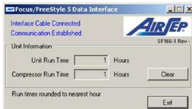
8. You may now record the hours from the Unit Run Time box. When recorded, turn the AirSep Focus off, disconnect AC power, disconnect data cable, and re-assemble.
