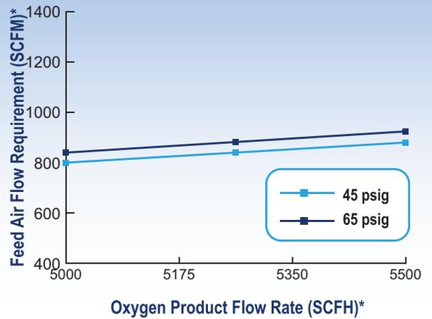
\* SCF (Standard cubic foot) gas measured at 1 atmosphere and 70°F
