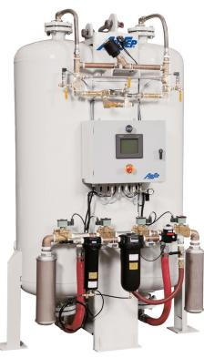
AirSep Alpha Series Nitrogen Generators produce from 450 to 46,905 cubic feet of nitrogen per hour at 99.5% nitrogen concentration. When electricity and an adequate source of compressed air is supplied, these dependable machines can provide nitrogen for practically any application and at concentrations up to 99.999% (10 PPM O2).
