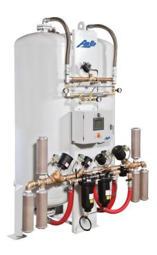
AirSep Alpha Series Nitrogen Generators produce from 450 to 46,905 cubic feet of nitrogen per hour at 99.5% nitrogen concentration. When electricity and an adequate source of compressed air is supplied, these dependable machines can provide nitrogen for practically any application and at concentrations up to 99.999% (10 PPM O2).
