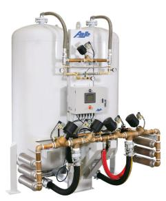
AirSep Alpha Series Nitrogen Generators produce from 450 to 46,905 cubic feet of nitrogen per hour at 99.5% nitrogen concentration. When electricity and an adequate source of compressed air is supplied, these dependable machines can provide nitrogen for practically any application and at concentrations up to 99.999% (10 PPM O2).
