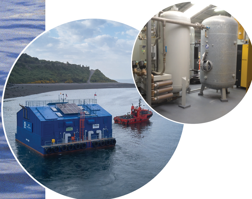
An AS-P2000 PSA Oxygen Plant (Oxymar® by OXZO S.A.) is used to provide oxygen for salmon fish farming sea cages in Chile.
