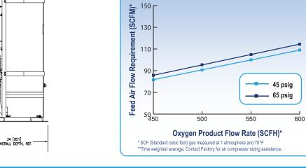
**Model AS-J Oxygen Generator** Feed Air Requirement\*\*
