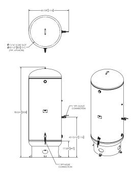
Model AS-L (flows above 1,199 SCFH) Generator 400 Gallon Oxygen Receiver
