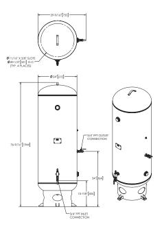
Model AS-G and AS-J Generator 120 Gallon Oxygen Receiver
