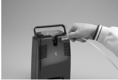
Figure 10: Connecting Cannula to FreeStyle 5's Oxygen Outlet
