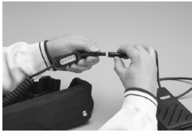
Figure 8: AirBelt Battery Charging
