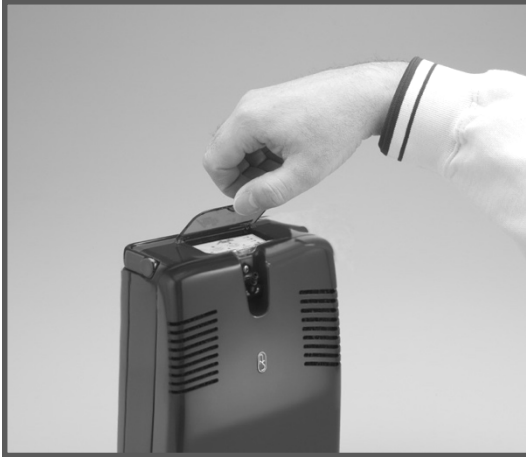
Figure 16: Lifting Dust Cover on Keypad Display
