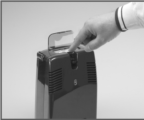
Figure 17: Pressing Flow Selection Button
