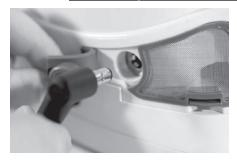
2. Connect the AC power cord to the AC power brick.
