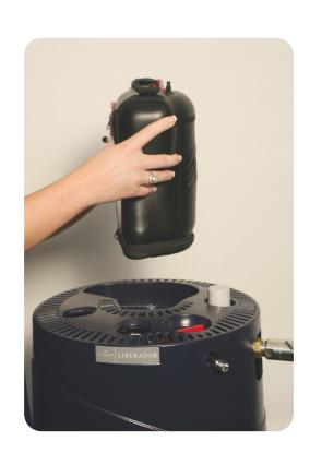
Turn the FCV to the zero position while filling. Position the portable unit above the reservoir's Quick Disconnect Valve and align it with the indentation on top of the reservoir. Press down on top of the portable unit to engage with the reservoir's Quick Disconnect Valve. Once the portable unit is engaged with the reservoir it can be filled.
