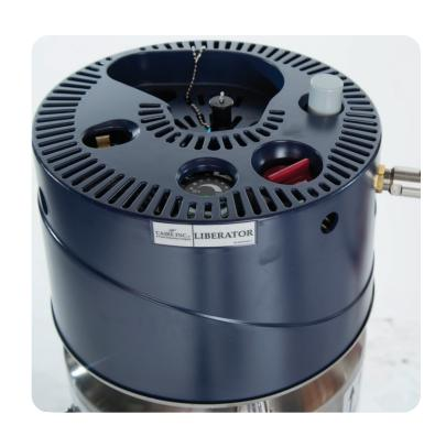
Clean the reservoir and portable unit fill connections to remove moisture and other contaminants with a lint free cloth. Do not disturb or depress the poppet on the reservoir or portable while drying the fill connectors. Also, be sure to keep the portable in the upright position at all times while wiping its fill connector.
