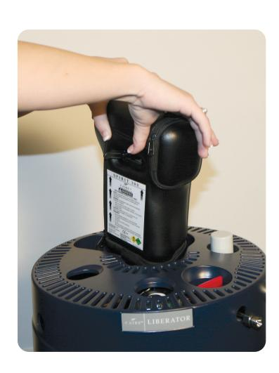
The unit is full when the hissing sound changes in tone and a dense, white vapor is seen coming from under the shroud of the reservoir. When this is observed, close the vent valve by raising its lever.
