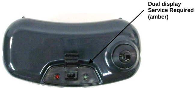
Figure 22: Indicator of Required Inspection/Service
