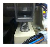
If replacement parts are necessary for an Integra utilizing conical springs, a kit is available that contains all the spare parts required to completely mount the compressor. This kit is part number #SP2670-SEQ and it contains 4 conical springs, 4 mounting bolts, 4 Neoprene washers, 4 metal washers, 2 compressor mount covers, and 2 screws for the mount covers.
