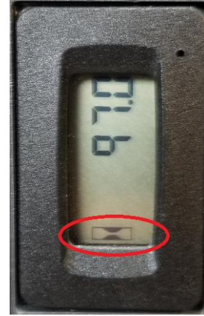
Figure 3. VisionAire™ and NewLife® hour meter
