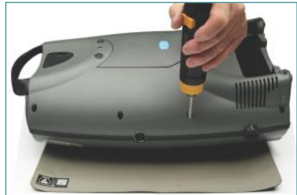
Figure 5. Removing or Installing Eclipse® Back Case
