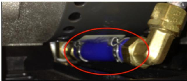
PN TU203-2 - NewLife Intensity 8 & 10 Fittings/Tubing connecting compressor to valve block.
