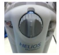
A: The HELiOS Marathon must detect a breath to begin delivering both demand and continuous flow. No flow will be delivered until a breath is sensed through the bottom cannula barb. A dual-lumen cannula must be connected to the Marathon and a patient must begin breathing before the flow will start.
