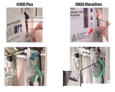
The purpose of this restriction is to slow the flow of liquid oxygen into the Marathon during a fill. This slower fill will aid to stabilize the pressure inside of the unit, and will allow it to be used properly almost immediately after a fill (within 15 minutes).
