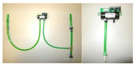
New NewLife® Elite O2 Monitoring board (Left) and NewLife® Intensity O2 Monitoring board (Right)
