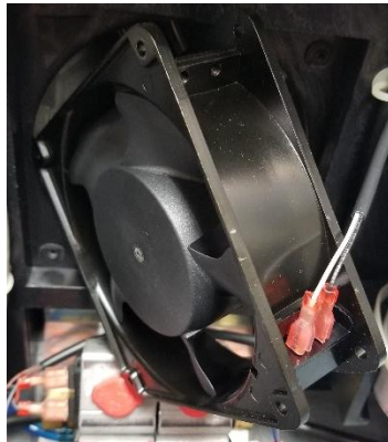
Figure 15.A. Installed Terminals to Fan
