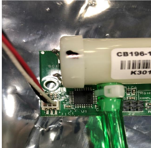
Figure 7. Connected Wire Harness and Tubing
