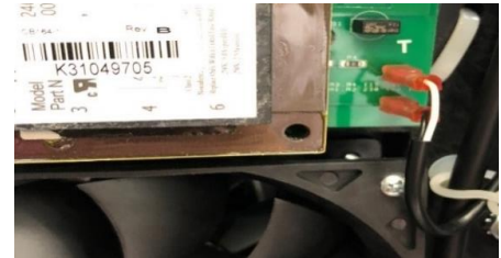
Figure 15.B. Installed Terminals to Fan Board
