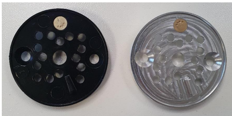
Left: old plastic lock plate. Right: new aluminum lock plate.
