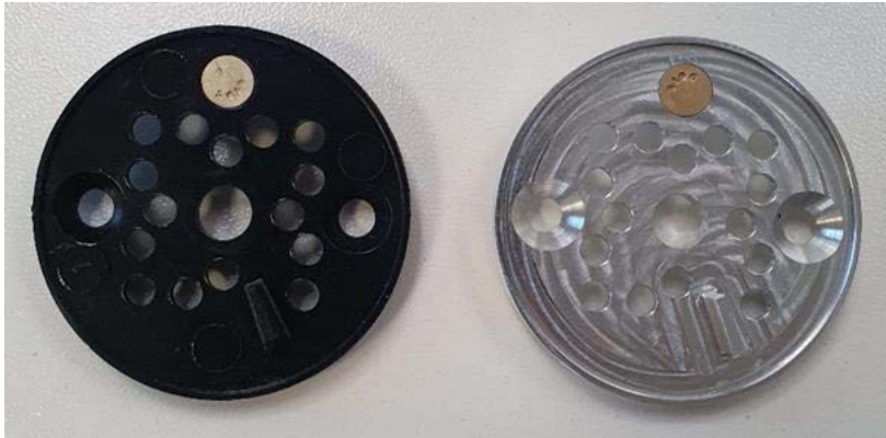
Figure 1 - Left old plastic lock plate. Right new aluminum lock plate
