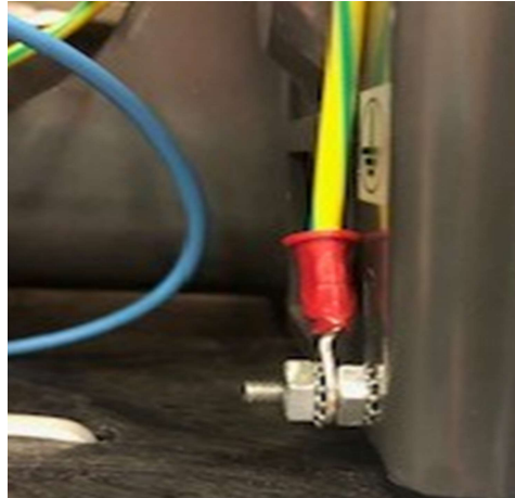
Figure 7. Ground wire and nut is located.
