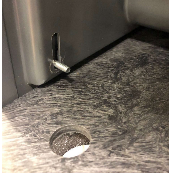
Figure 11. Shows the screw on the front panel once the nut is removed.
