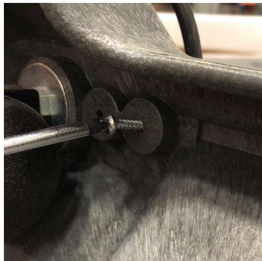
Figure 10. Location of two Philips head screws on the bottom of the base of the unit.
