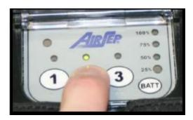
b) Press and hold the selector buttons 1 and 3 simultaneously until the audible tone sounds (For the FreeStyle® 5 press and hold 1 and 5)
