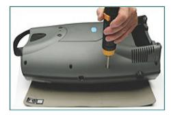
Figure 1 - Eclipse Removal and Installation of Screws
