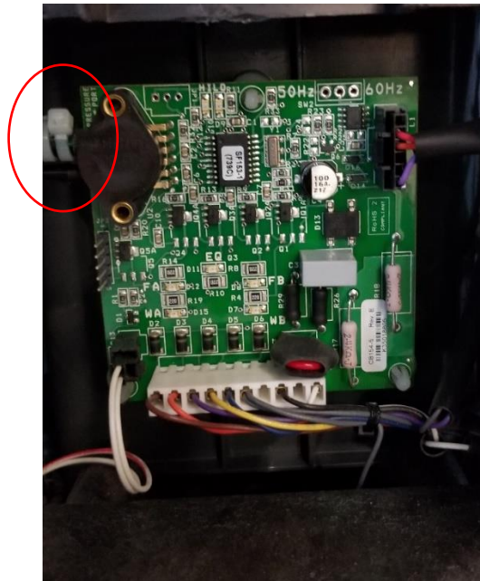
Figure 3. Pressure Transducer Zip Tie
