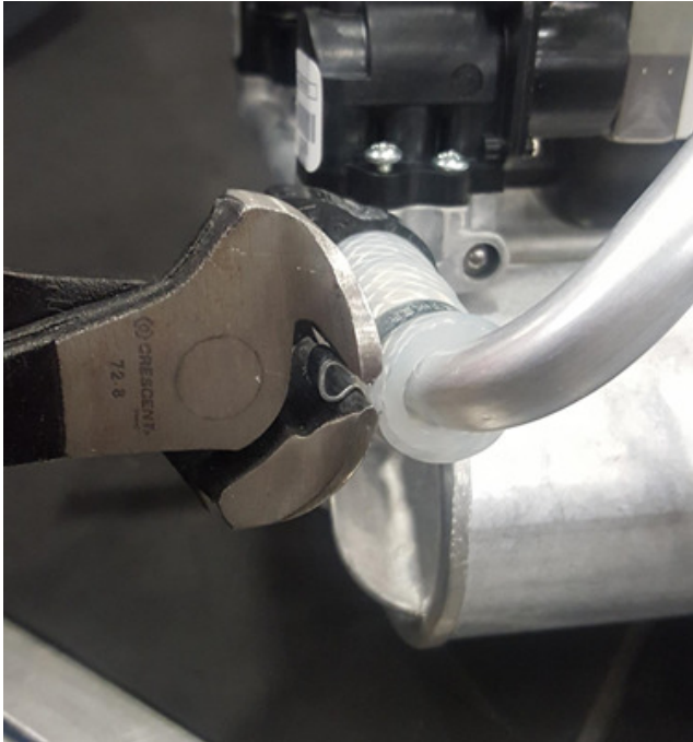
Fig. 5: Crimping Pinch Clamp
