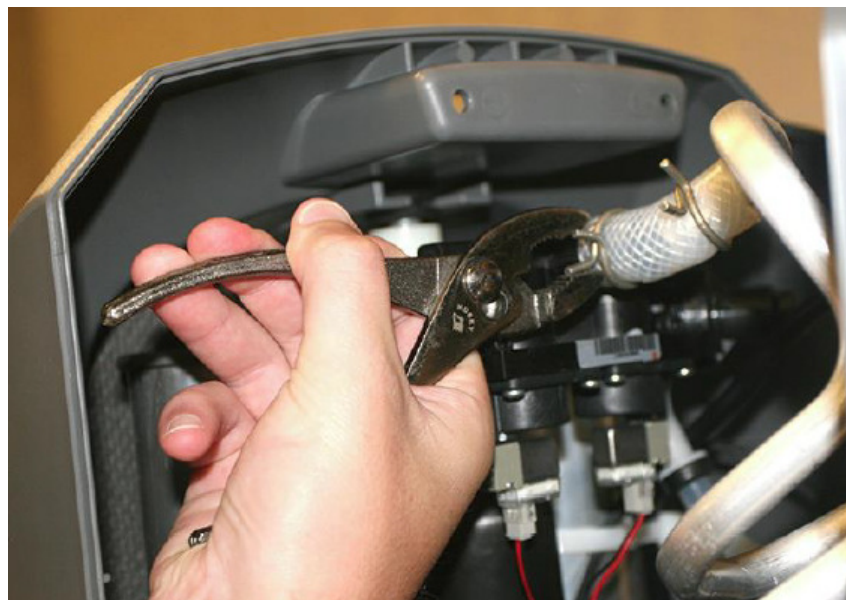
Fig. 4: Previous Design Clamp Removal
