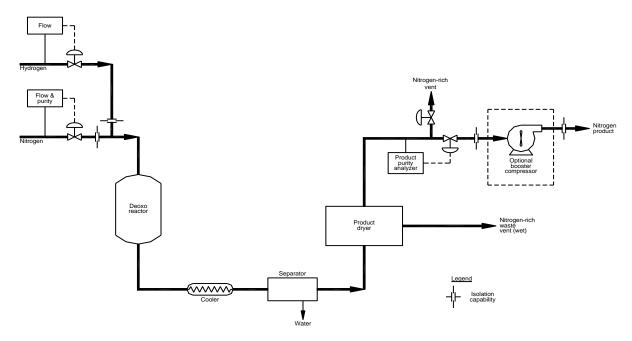
Figure 14 Typical deoxo flow diagram
