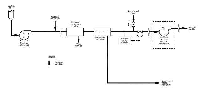
Figure 11 Typical membrane nitrogen flow diagram
