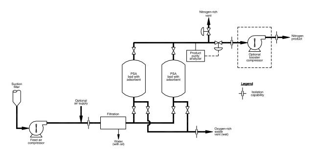
Figure 7 Typical PSA nitrogen generator flow diagram
