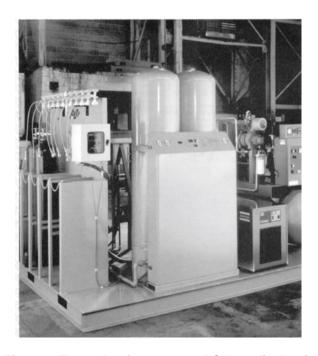
Figure 6 Example of an oxygen PSA medical unit
