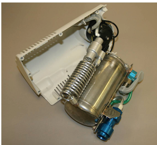
Figure 25: H300 Container Removal
