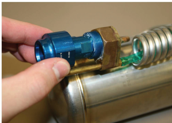
Figure 43: H850 QDV Removal
