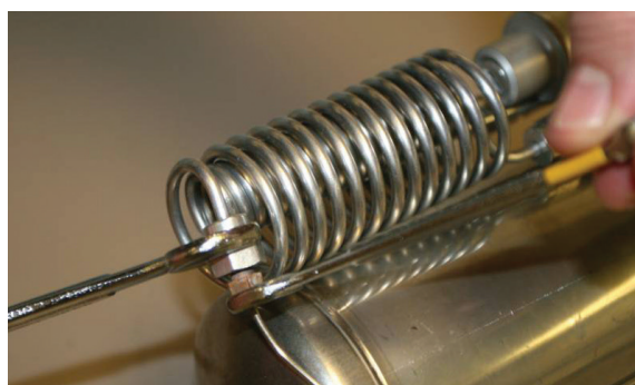
Figure 33: Compression Nut Removal
