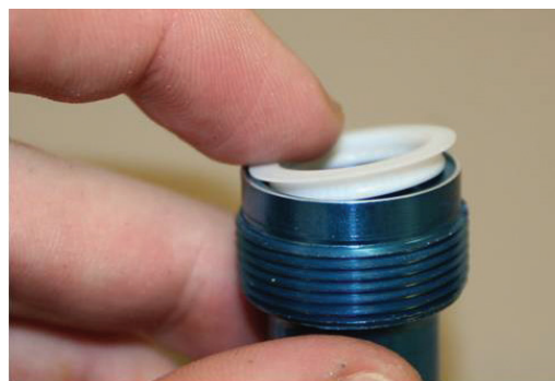
Figure 45: Lip Seal Replacement
