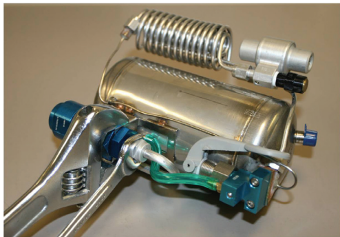
Figure 40: H300 QDV Removal
