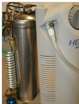
Figure 20: Pressurizing the HELiOS Portable
