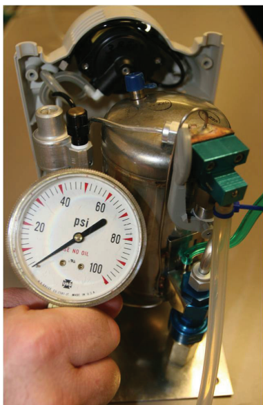
Figure 28: Test Pressure Gauge Set-Up
