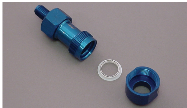
Figure 44: Lip Seal Removal
