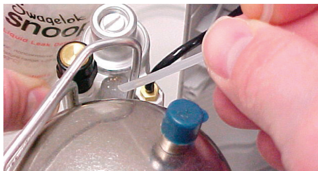
Figure 29: PRV Liquid Leak Testing
