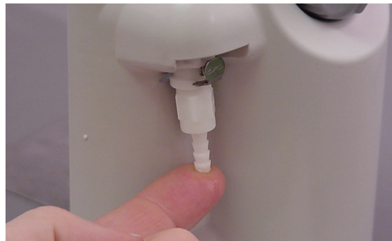
Figure 22: Inline Check Valve Leak Test
