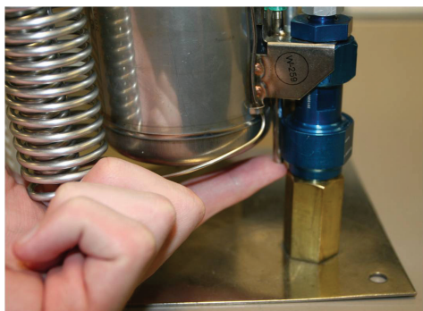
Figure 21: Vent Outlet Leak Testing
