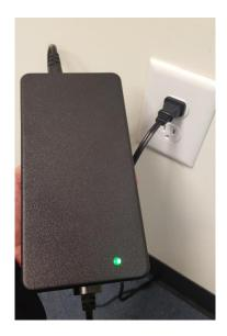
NOTE: The AC power cord cannot plug directly into Power Receptacle on side of the Eclipse 5. Doing so will damage the unit.
