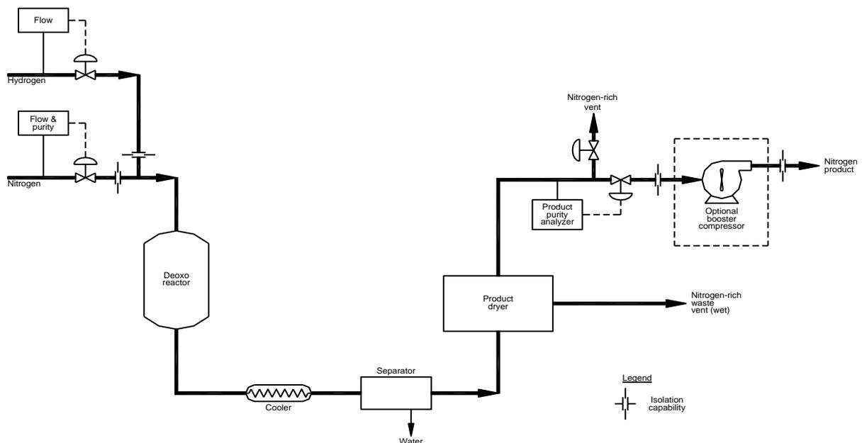
Figure 14 Typical deoxo flow diagram
