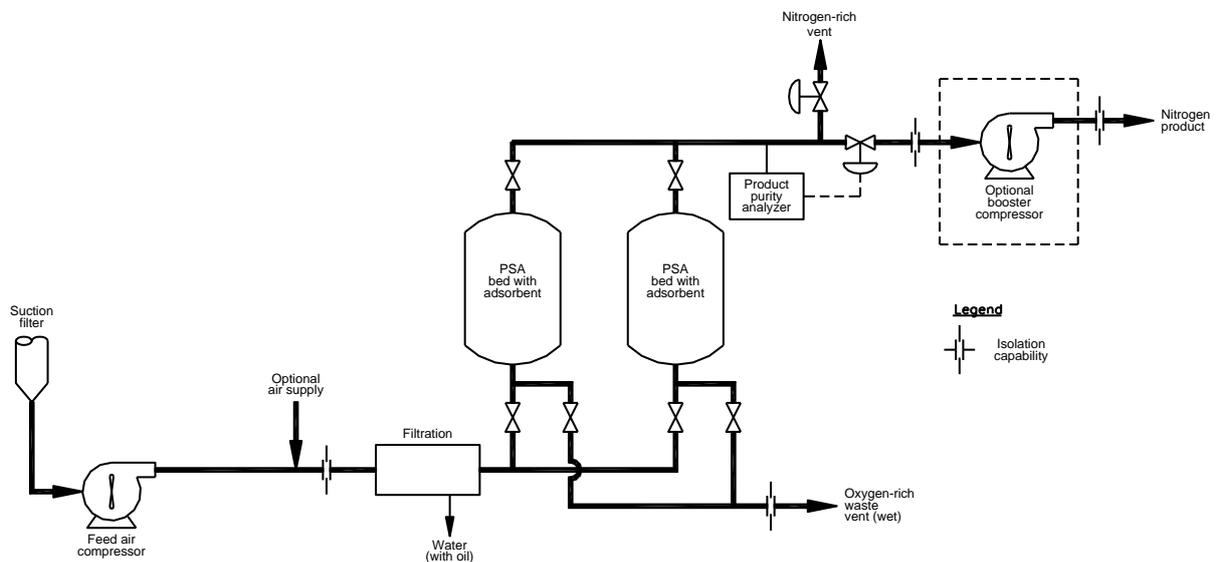
**Figure 7 Typical PSA nitrogen generator flow diagram**
