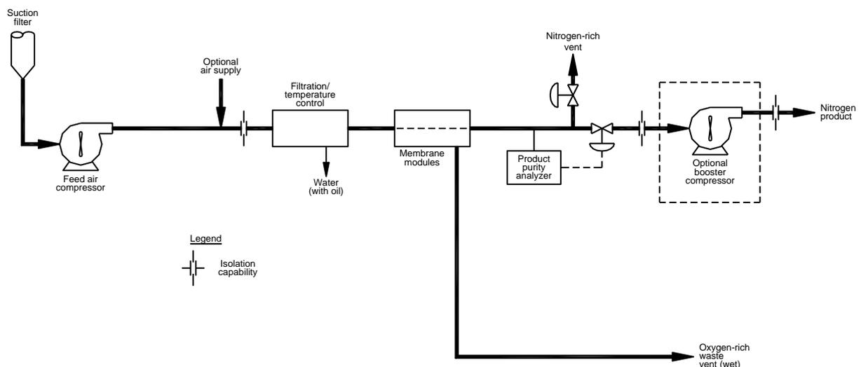
**Figure 11 Typical membrane nitrogen flow diagram**
