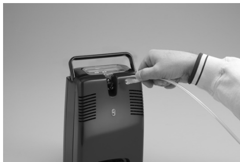
Figure 10: Connecting Cannula to FreeStyle 5's Oxygen Outlet
