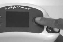
A brief audible alarm will sound to indicate the device has powered on.
