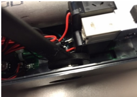
Use 13 mm wrench to attach harness to Freestyle
