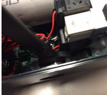
Use 13 mm wrench to remove harness
