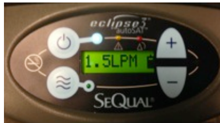
Power Cartridge Status Gauge Location for Eclipse 3 (right side of green illuminated display)
