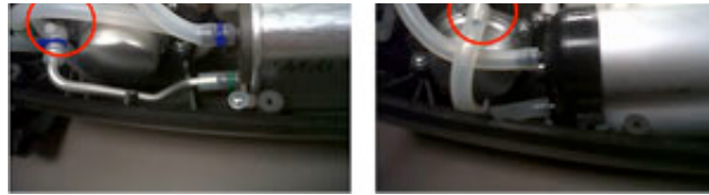
Figure 5--ATF Outlet Location for Tubing Connection
