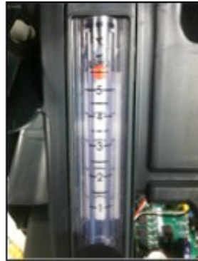
Flow Meter with Ball at 5.5 LPM
