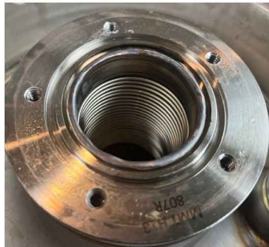
Old style bellows neck tube design
