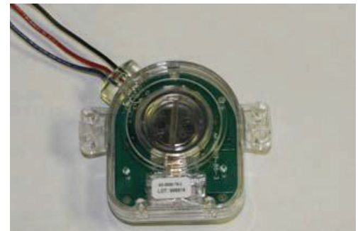
Figure 2: Back of G4 liquid level gauge.
