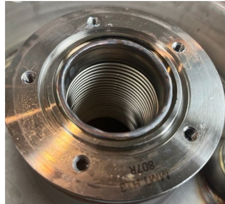
Old style bellows neck tube design
