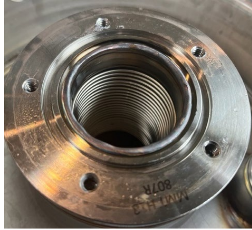
Old style bellows neck tube design
