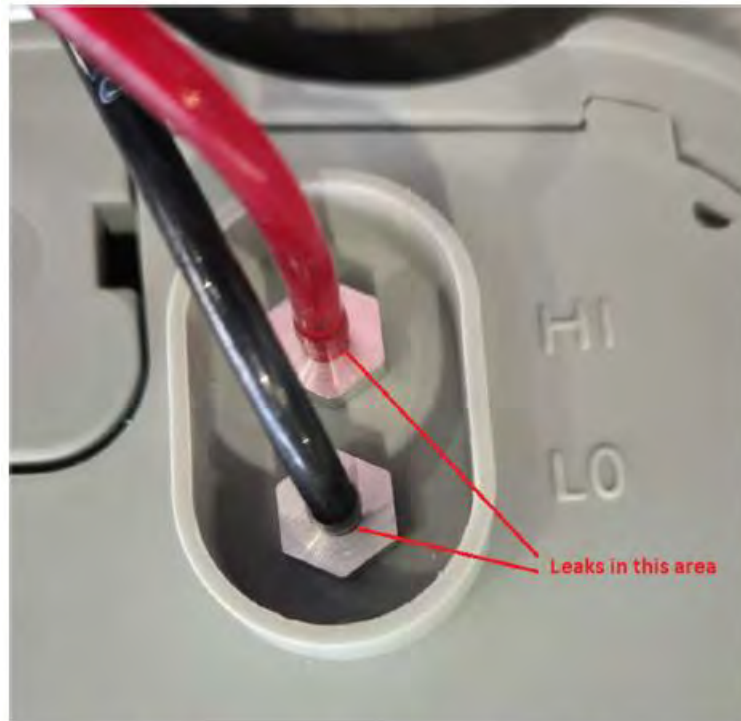
Figure 1 – Area where leaks may occur
