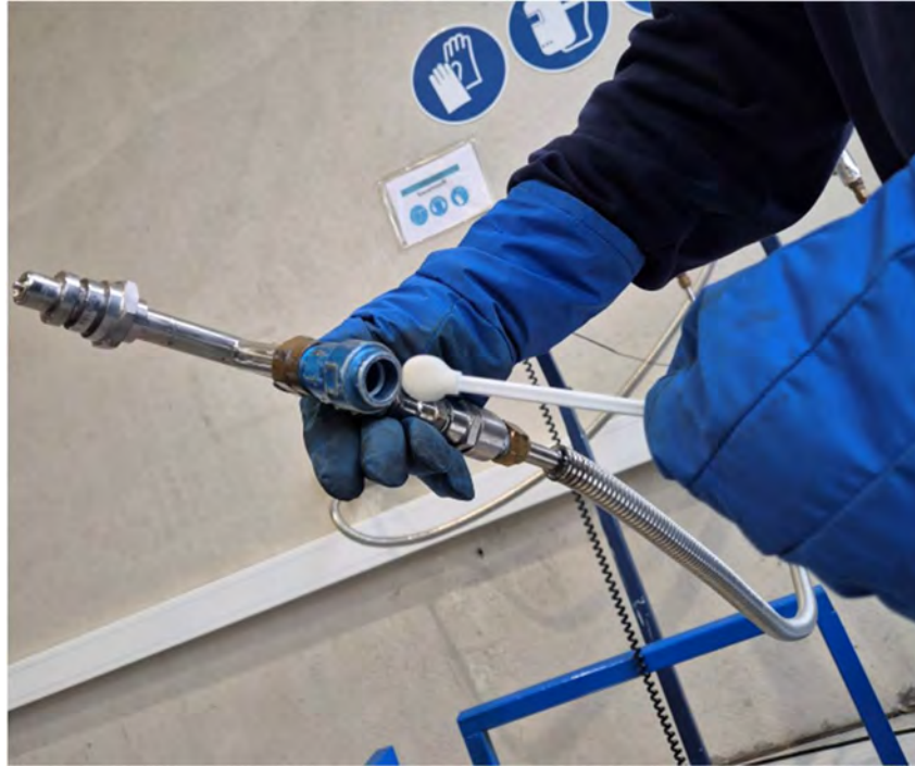
Figure 7 – Wiping of fill connectors depending on QDV Fitted.
