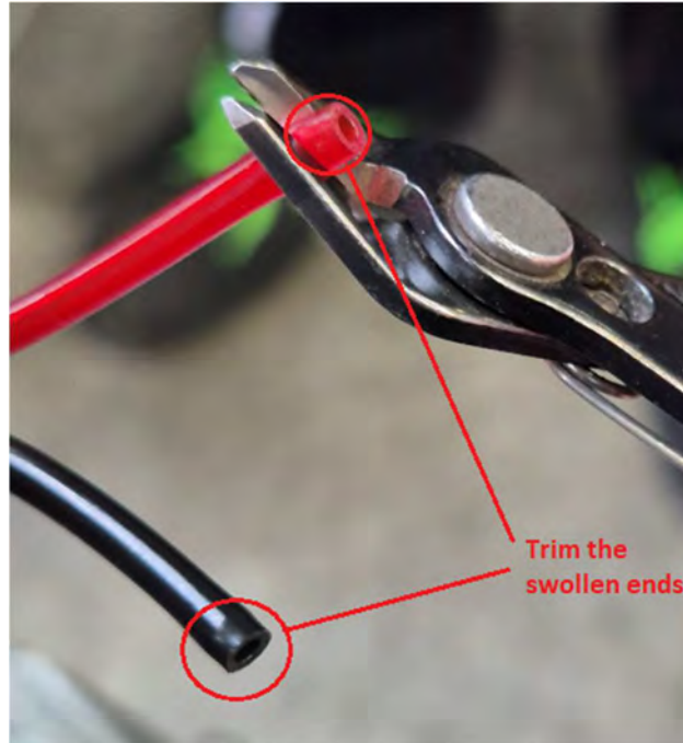
Figure 2 – Trim tubing 3/8" (9mm)
