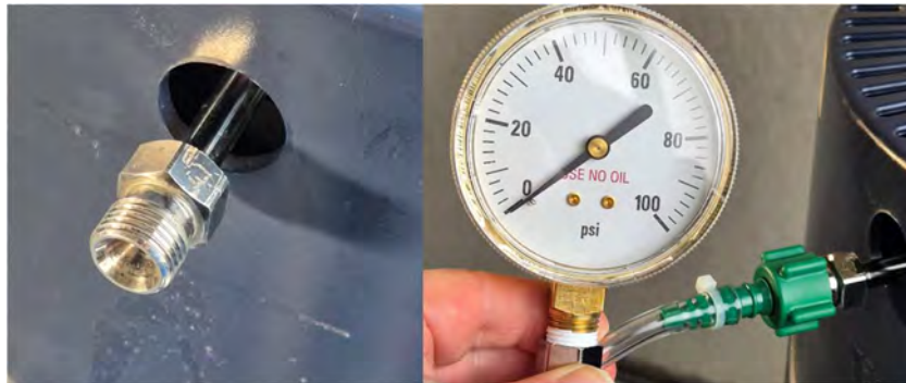
Figure 8 – FCV extension fitted to FCV and pressure gauge to FCV extension.
