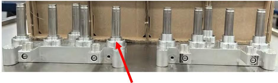
Left side manifold shows a longer stem and a reduction on the valve seating.
