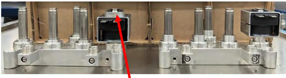
Left side manifold shows valve fitted with washer HA197-1 and secured with clip.
